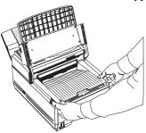
3. Pull the colored lever on the old toner cartridge all the way toward you. Carefully pull the old toner cartridge out of the
